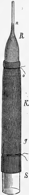
FIG. 478.—Apparatus for illustrating the change in the turgidity of cells caused by external distension or compression.
